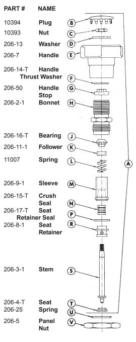
(A) Bonnet Assembly (206-102-1) Consists of all functional parts, sealed and ready to install in body
