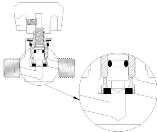
Robbins seats are fully contained inside the cup of the bonnet and the body of the valve.
